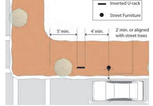
Figure 7-24 Inverted U-Rack spacing recommendations
