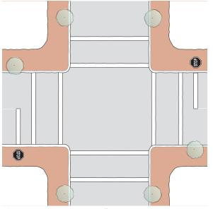
Figure 7-27 Transverse crosswalk striping
