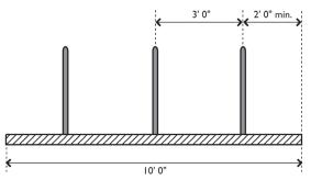
Figure 7-25 Inverted U-Rack spacing recommendations
