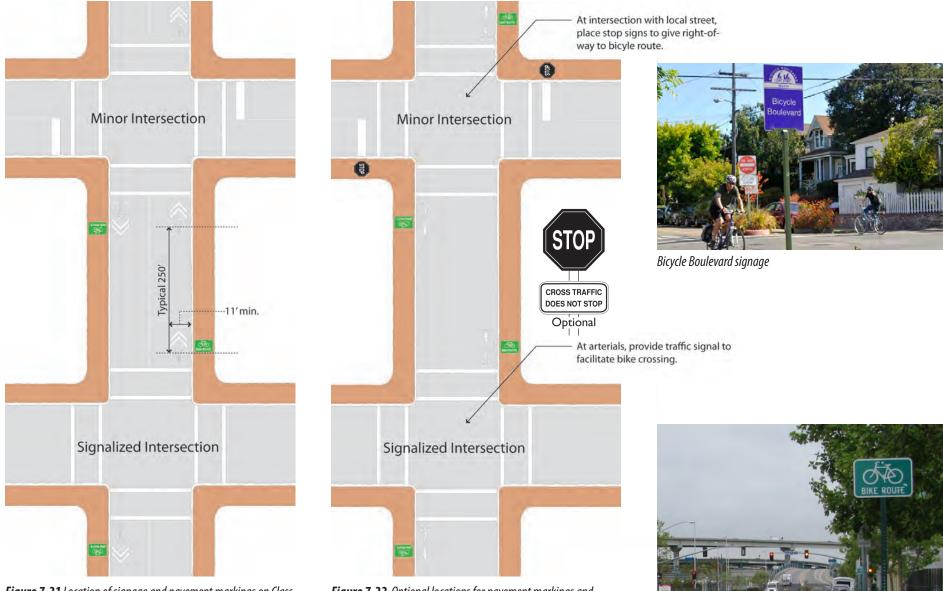
*Figure 7-21* Location of signage and pavement markings on Class III bike route
