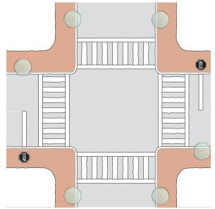
Figure 7-28 Ladder crosswalk striping
