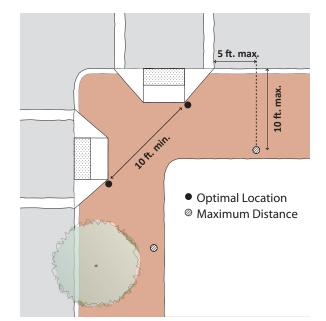
*Figure 7-36 Recommended installation for accessible pedestrian signals*
