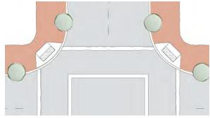
**Figure 7-38** Larger Turning Radii - widen pedestrian crossing and limit amount of sidewalk available for perpendicular curb ramps
