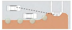
*Figure 7-30 Improved visibility - Curb extensions can help improve pedestrian visibility*
