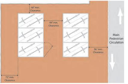
*Figure 7-26 Bicycle locker placement requirements*
