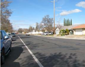
**Top** Yolo Street is designated as a Class II bikeway but is not striped or signed to meet Caltrans Standards. **Above** Bicycle/parking lanes on Balsam Drive, letting cars encroach onto the bicycle right-of-way.
