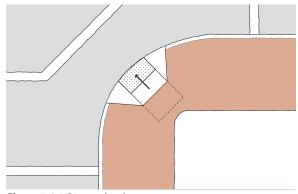
Figure 7-34 Diagonal curb ramp
