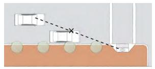
*Figure 7-29 Limited visibility – Parking too close to an intersection can hinder pedestrian visibility*
