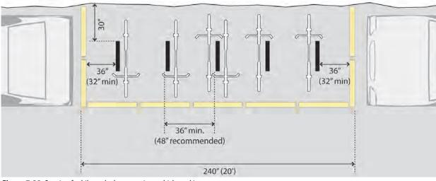
*Figure 7-23 Spacing for bike rack placement in a vehicle parking space*
