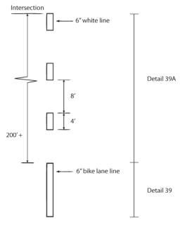
Figure 7-4 Class II bike lane striping detail
