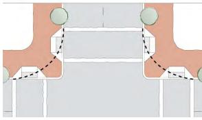
*Figure 7-39 Smaller Turning Radii - reduce the pedestrian crossing distance and create more sidewalk room for perpendicular curb ramps*
