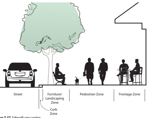
Figure 7-37 Sidewalk cross section
