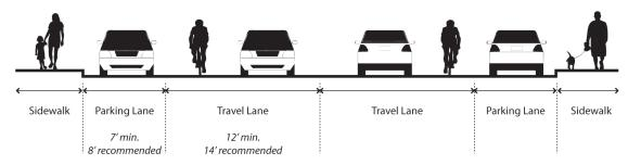
*Figure 7-15* Class III bike route cross section
