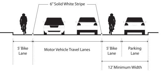
*Figure 7-3 Class II bike lane cross section adjacent to curb and gutter and adjacent to parallel parking*
