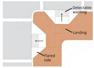
*Figure 7-32 Perpendicular curb ramps - preferred*
